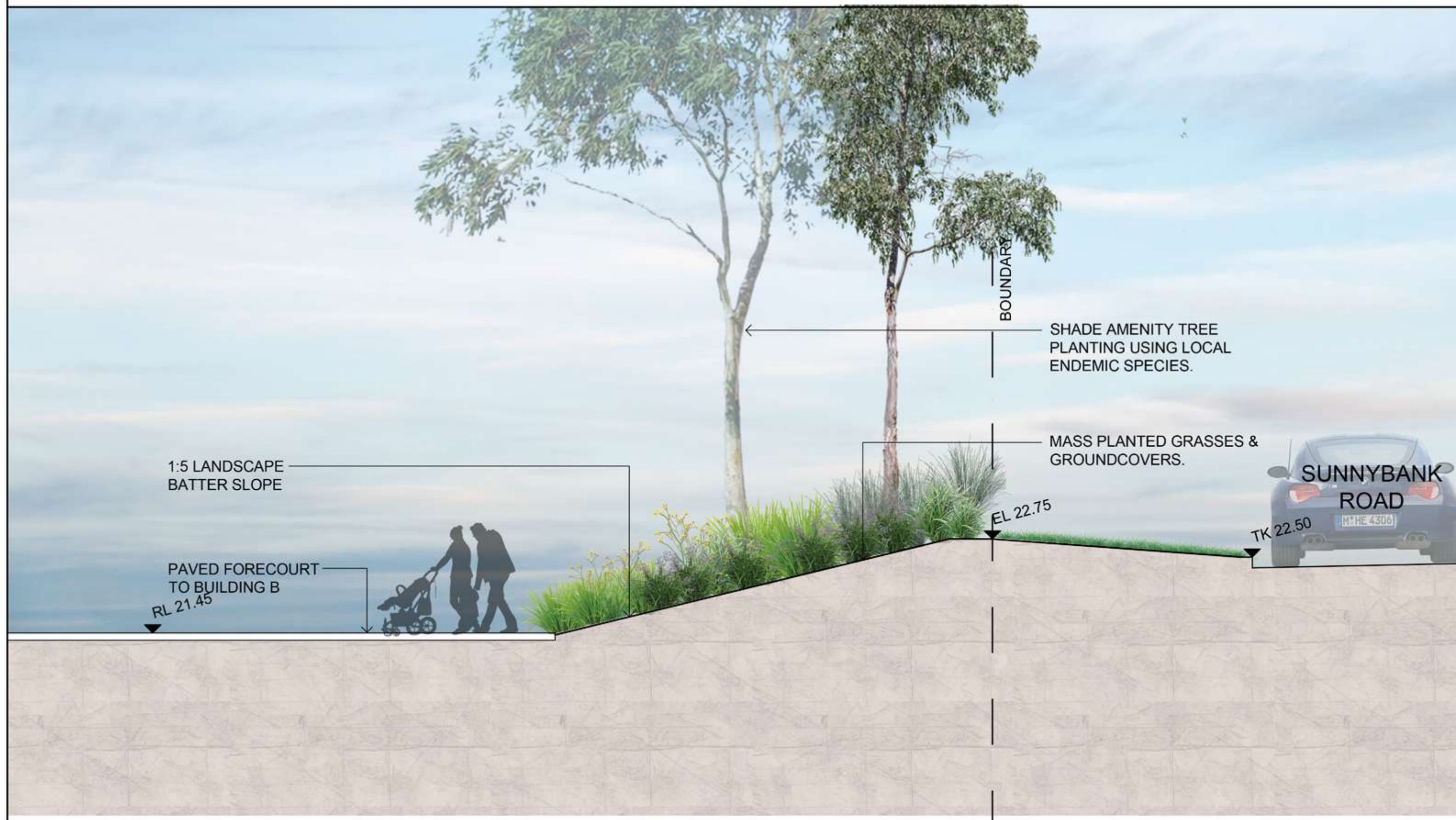
02 SECTION FF 602 SCALE 1:50
