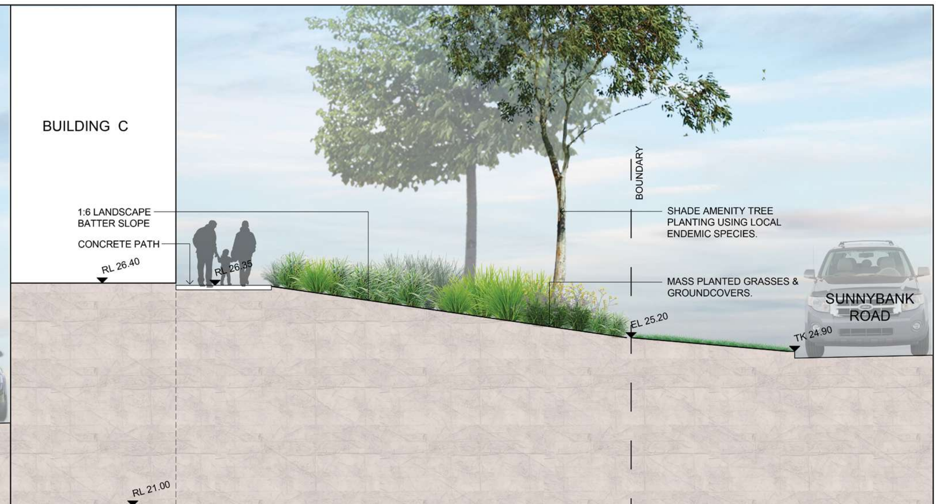
03 SECTION GG 602 SCALE 1:50
